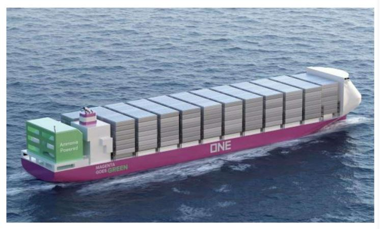
ONE has received design approval in principle for a dual-fuel 3,500-TEU ship capable of being powered by ammonia, a colorless chemical that emits no CO2 when burned. Photo credit: ONE.
